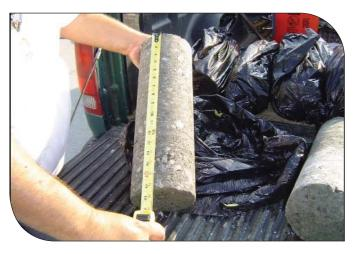
Quality control check using pavement cores after 7 days.
