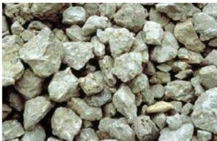
Figure 121. Recycled concrete aggregate (source: Jonathan Gene Pitre, University of New Hampshire)
