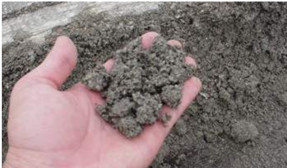
Figure 120. Typical concrete pavement millings from milling operation (source: Dan DeGraaf, Michigan Concrete Paving Association)
