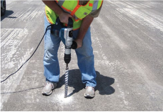
Figure 8. Hammer drilling to check pavement thickness
