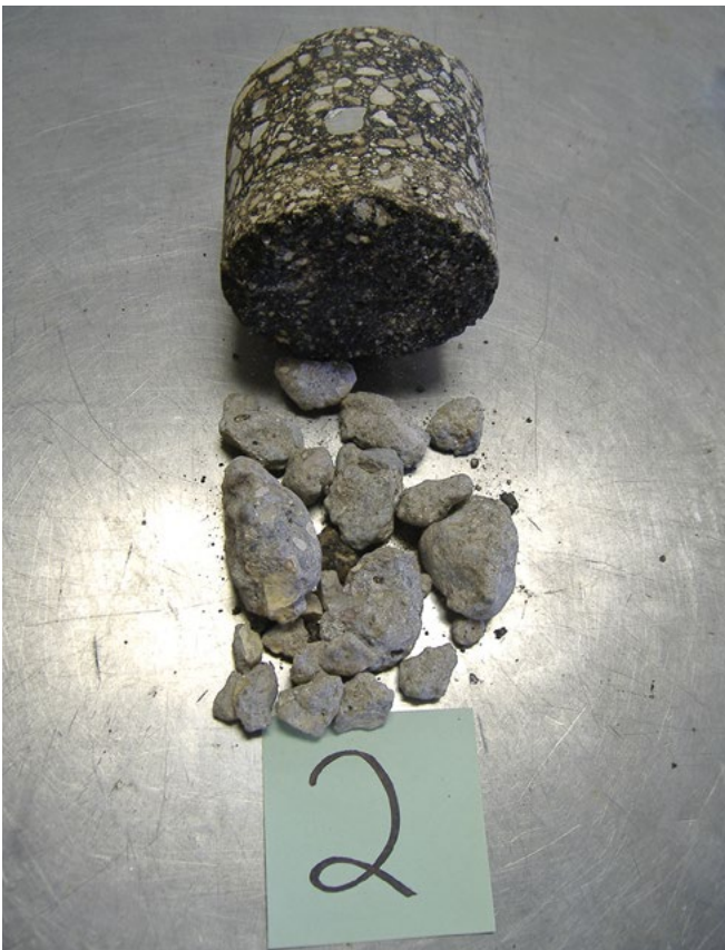
Figure 9. Typical core of asphalt parking lot with granular subbase
